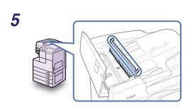
Clean the transparent plastic part of the inner cover with a water-moistened cloth. Then, wipe the area with a soft, dry cloth.
